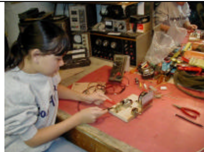
Here I am testing the current limiting resistor with a volt-ohm meter.
